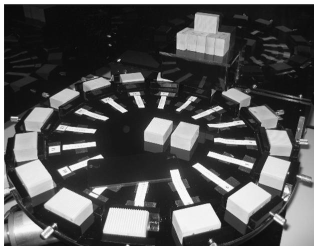
Fig. 1 – An overhead view of the Spinning Wheel for presenting tactile stimuli to the index fingertip.
